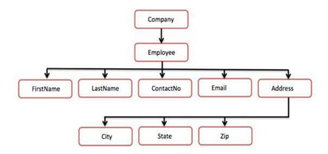
In the above diagram, there is a root element named as <company>. Inside that, there is one more element <Employee>. Inside the employee element, there are five branches named <FirstName>, <LastName>, <ContactNo>, <Email>, and <Address>. Inside the <Address> element, there are three sub-branches, named <City> <State> and <Zip>.
